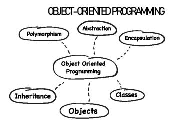
**Encapsulation** is the unity of data and methods to apply on data, which are shared both by classes and by objects. Data can only be accessed through the object which was designed to operate on that particular data (data are hidden from manipulation). This feature is also called **information hiding**.
